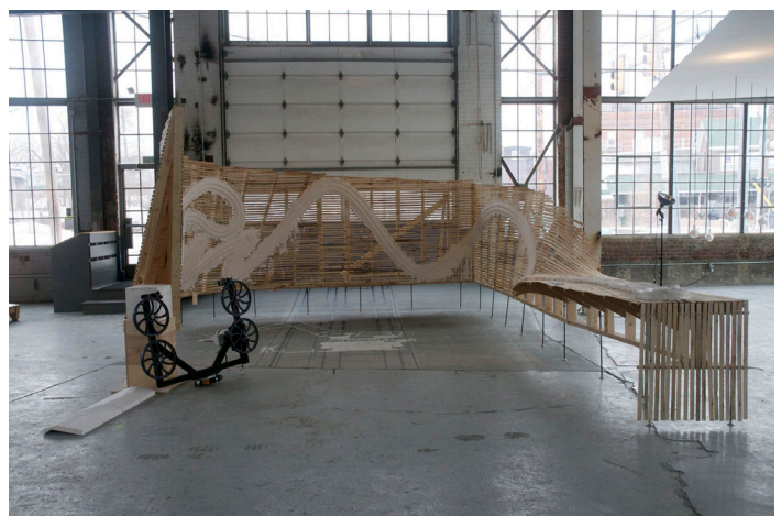
Figure 1. Morphfaux demonstration construct, robotically profiled plaster on bentwood lath.
