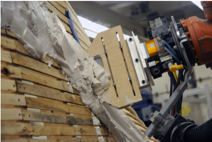
Figure 2. Plaster compensating for the difference in digital model and real wood construct.
